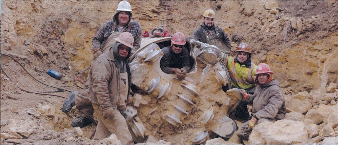
LEFT: The Robbins 72-inch (1.8 m) Motorized SBU (SBU-M) broke through almost exactly on line and grade after 395 ft (120 m) of boring. RIGHT: The Robbins SBU-M was the largest machine of its kind ever made, and utilized a mixed ground cutterhead in clays as well as rock.
